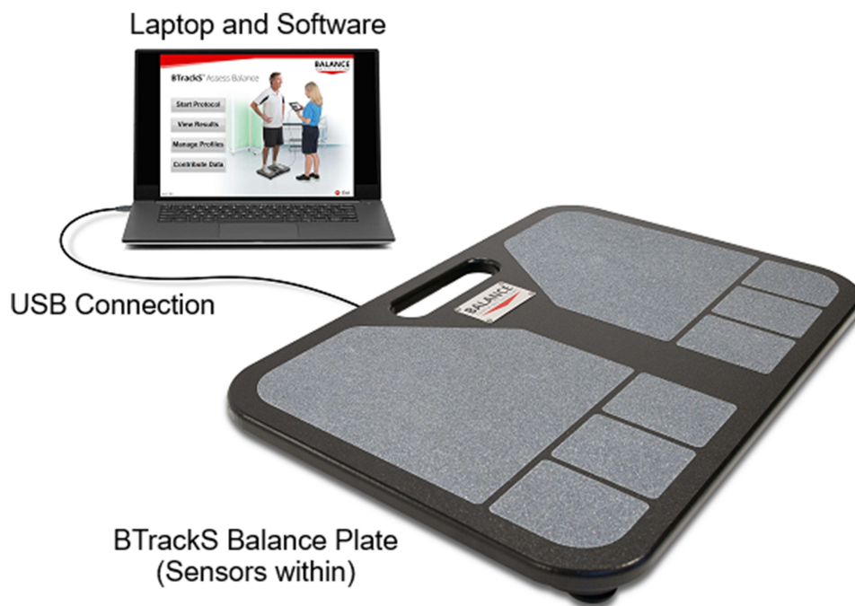
Figure 2 The Balance Tracking System (BTrackS) Balance Plate and software running on a laptop computer.
